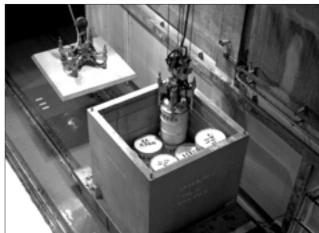
The El Cabril site in Spain: the drums of radioactive waste are introduced into the concrete container before being disposed of into the repository vaults.
